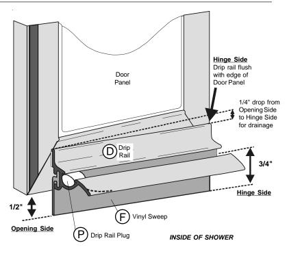
Drip rail may be additionally secured using 8A x 3/8" truss head screws. When drilling in door panel, make certain drill does not hit glass. Glass is seated approximately 1/2" into channel.
